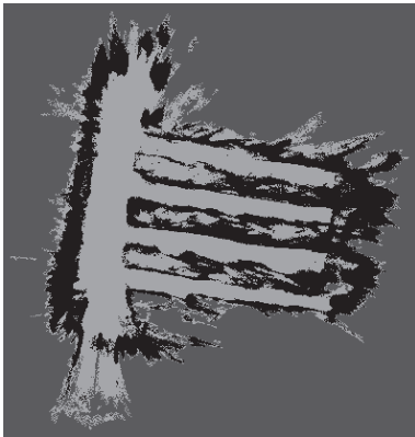
Fig. 7: Occupancy grid map generated by RTAB-Map
